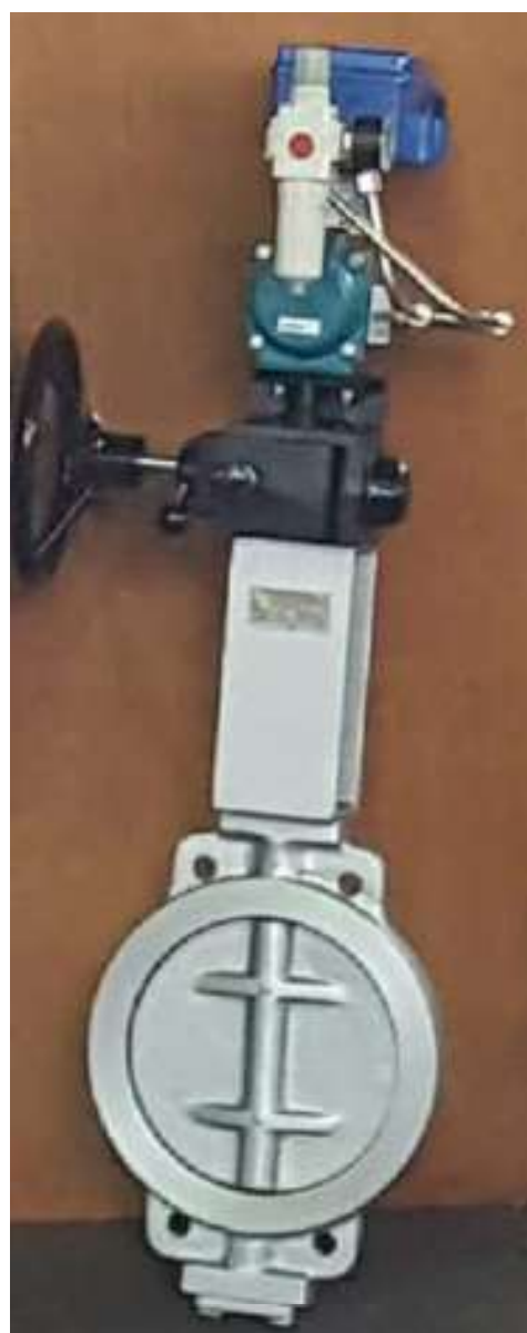
Valvola a farfalla damper DN 150 Corpo e disco in ghisa HT - Forata PN 6 Tipo wafer Damper butterfly valve DN 150 Body and disc in cast iron HT - Drilled PN 6 Wafer type
