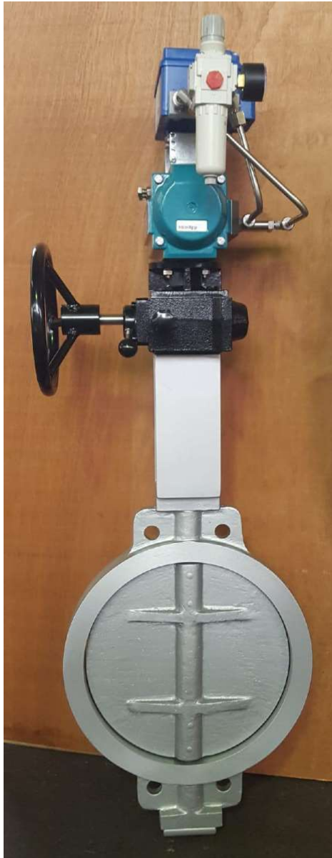
Valvola a farfalla damper DN 300 Corpo e disco in ghisa HT - Forata PN 6 Tipo wafer Damper butterfly valve DN 300 Body and disc in cast iron HT - Drilled PN 6 Wafer type
